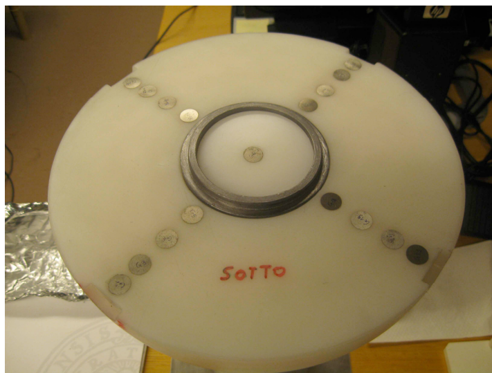
Fig. 1. Schematic view of the spectrometer showing the arrangement of the activation foils detectors along three perpendicular axes, as well as the inner lead layer.
